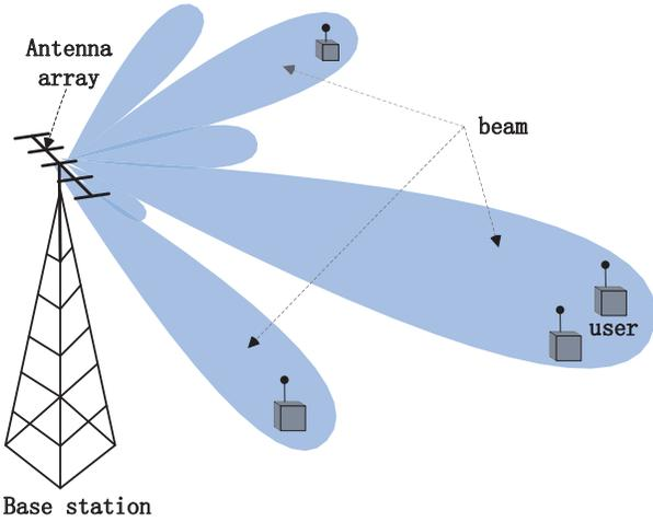
Fig. 1. System model. The base station equips antenna array. The shadows are the transmitting beams pointed to different users or users group.
