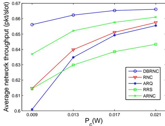
Fig. 2. Average network throughput vs. transmitting power
