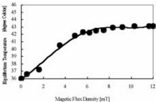
Fig. 3. Effects of the magnetic flux density on thermal equilibrium. The equilibrium temperature of the stent was nearly constant above 6 mT.
