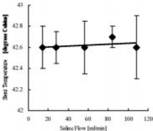
Fig. 4. Effects of the saline flow on the stent temperature. The saline flow was altered from 17 ml/min to 145 ml/min. The temperature remained nearly constant.
