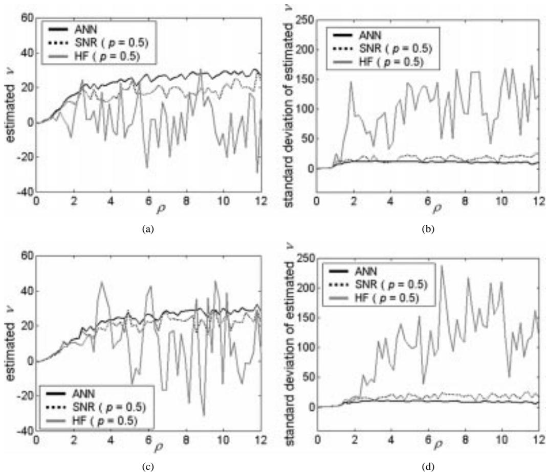
Fig. 4. Mean and standard deviation of  $\hat{\nu}$  for simulated echo envelopes. (a) Mean,  $N = 300$ . (b) Standard deviation,  $N = 300$ . (c) Mean,  $N = 625$ . (d) Standard deviation,  $N = 625$ .
