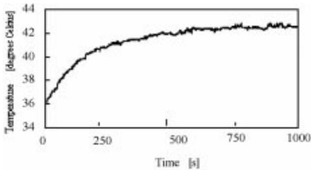
Fig. 2. The time required for temperature stabilization of the stent under 25-KHz magnetic field irradiation. The magnetic flux density was 10 mT, the circulating saline temperature was 36 °C when the flow was 58 ml/min, and the stent temperature was maintained at 42.6 °C thermal equilibrium.
