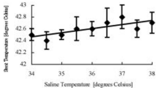
Fig. 5. Effects of the circulating saline temperature on the stent temperature. The temperature of stent rose gradually when the temperature of saline was increased from 34 °C to 38 °C. The temperature coefficient,  $\Delta T_{st}/\Delta T_{sa}$  was 0.05, where  $\Delta T_{st}$  was the stent temperature change, and  $\Delta T_{sa}$  the saline temperature change. The saline flow was 58 ml/min.
